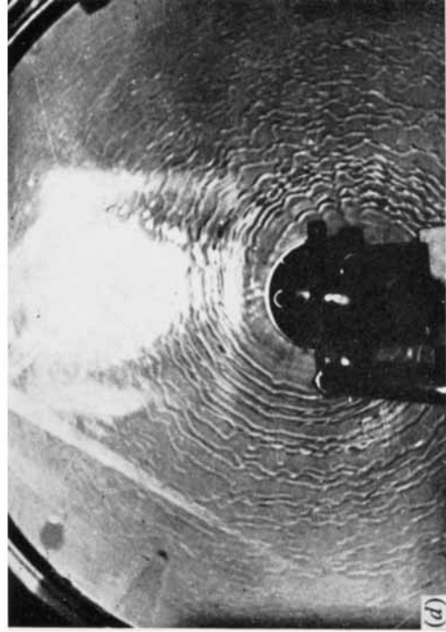
FIGURE 4. Examples of waves occurring on the surface of the disk Q (c.c./s) \omega' (rev/s) \sigma^* \nu^* (a) Smooth film 5 1 0.95 1.0 (c) Spiral waves 2.5 6 0.98 1.7 (b) Concentric waves 12 1 0.95 1.0 (d) Irregular break up of spiral waves 10.8 10 0.96 1.0
